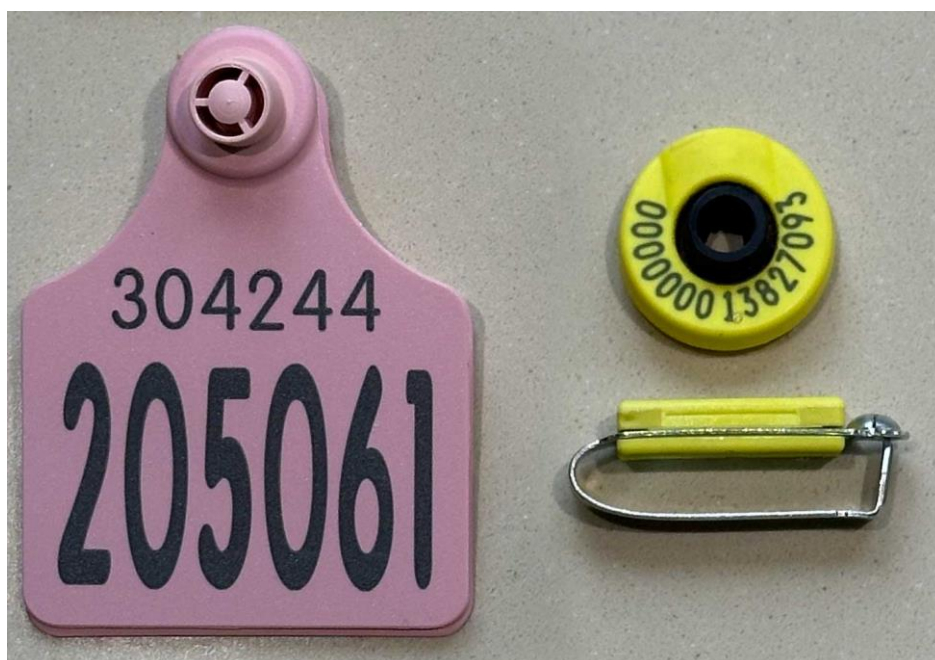
Figure 6.2. Comparative sizes of a UHF flag tag (left) with an LF button tag (upper right) and an LF metal tag (lower right). The UHF flag tag is 60mm wide (and should be about 1:1 scale at A4).
