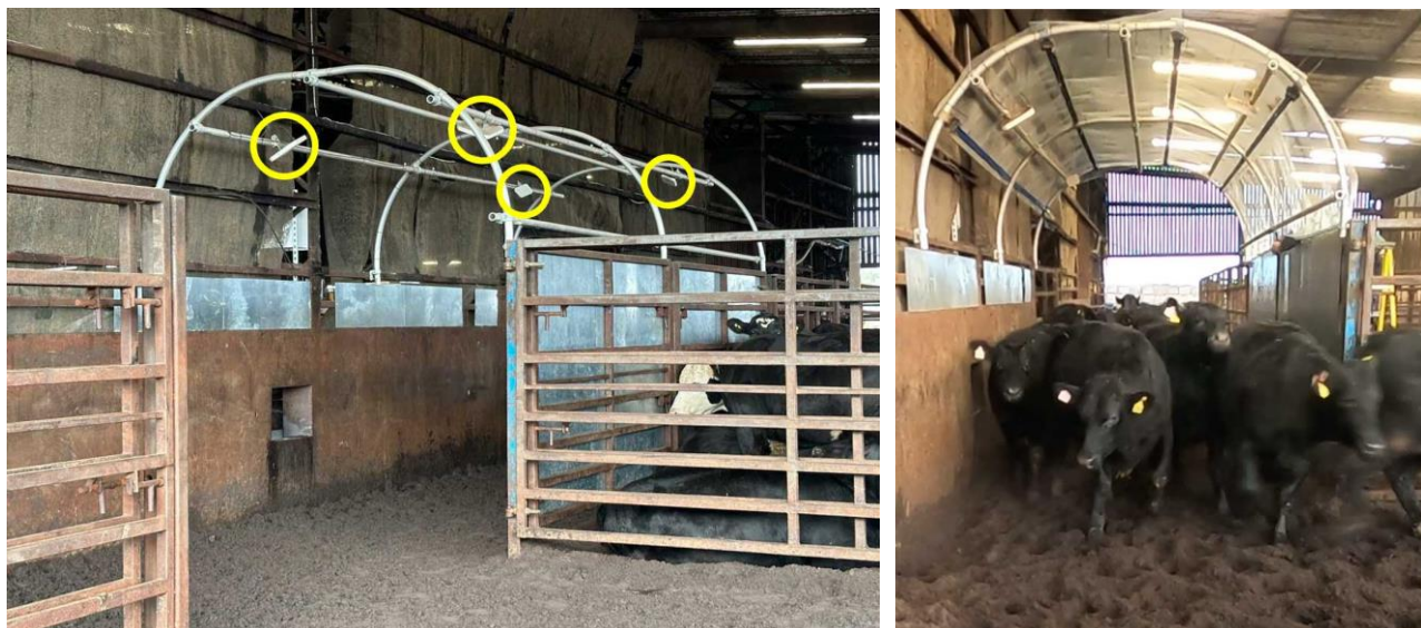
Figure 2.2. Photograph (left) showing the four UHF antennas (circled in yellow) above the 2.75m wide alleyway, and a video still (right) showing cattle moving under the UHF antennas during the trial. Note that wire mesh (visible in the still on the right) had been installed above the antennas after the photograph on the left was taken. This mesh is believed to help read tags in animals in the UHF ‘tunnel’, and reduce the risk of accidentally reading any animals adjacent to the tunnel.
