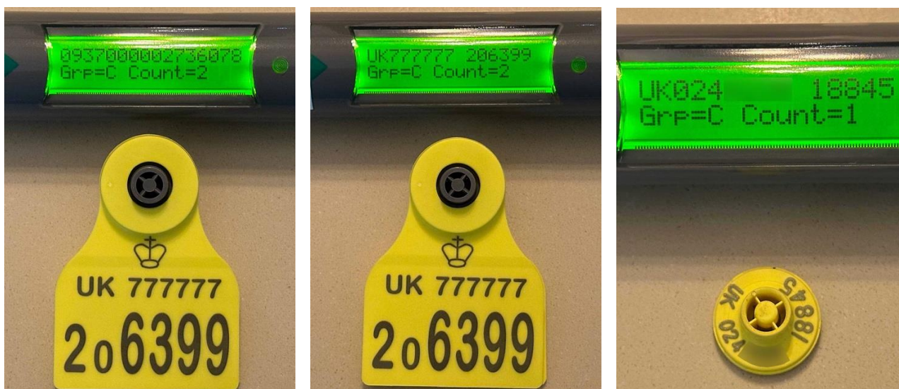
Figure 5.1. Before a tag bucket file is uploaded, LF stick readers can only display the 'random' number encoded on the chips currently used in LF cattle management tags (left). Once the tag bucket is loaded, the stick can display the corresponding VID i.e. the animal number as printed on the tag (centre). UK sheep LF EID tags are WYSIWYG which means the VID is programmed on the LF chip, and the stick can therefore display the VID without needing a tag bucket file (right).
