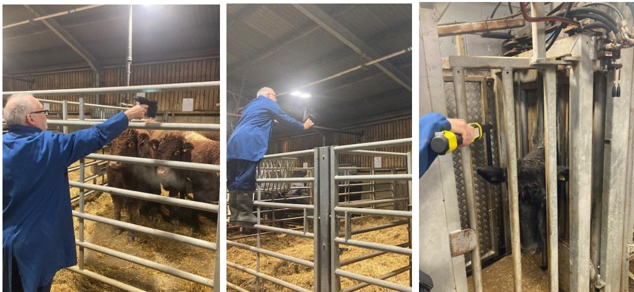
Figure 4.1. Photographs showing trial cattle being scanned with a hand-held UHF reader in the abattoir lairage (left and centre) and with an LF stick reader in the abattoir crush (right). Note that in the crush, the animal's neck is held in the head yoke to restrict head movements. This ensures that the LF stick reader can be used with minimal risk of injury to the operator. In practice, static EID readers (either UHF or LF) would be used in the crush, further reducing injury risk to operators, and could operate without the need to use the head yoke. The head yoke would still be used to restrain any animal requiring manual identification (when the EID tag is missing or not working).
