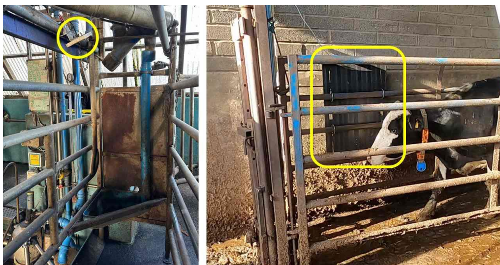
Figure 2.4. One of the UHF antennas in one of the eight milking stalls (left, circled in yellow), and the LF static panel reader (right, in the yellow box) on the narrow exit raceway.
