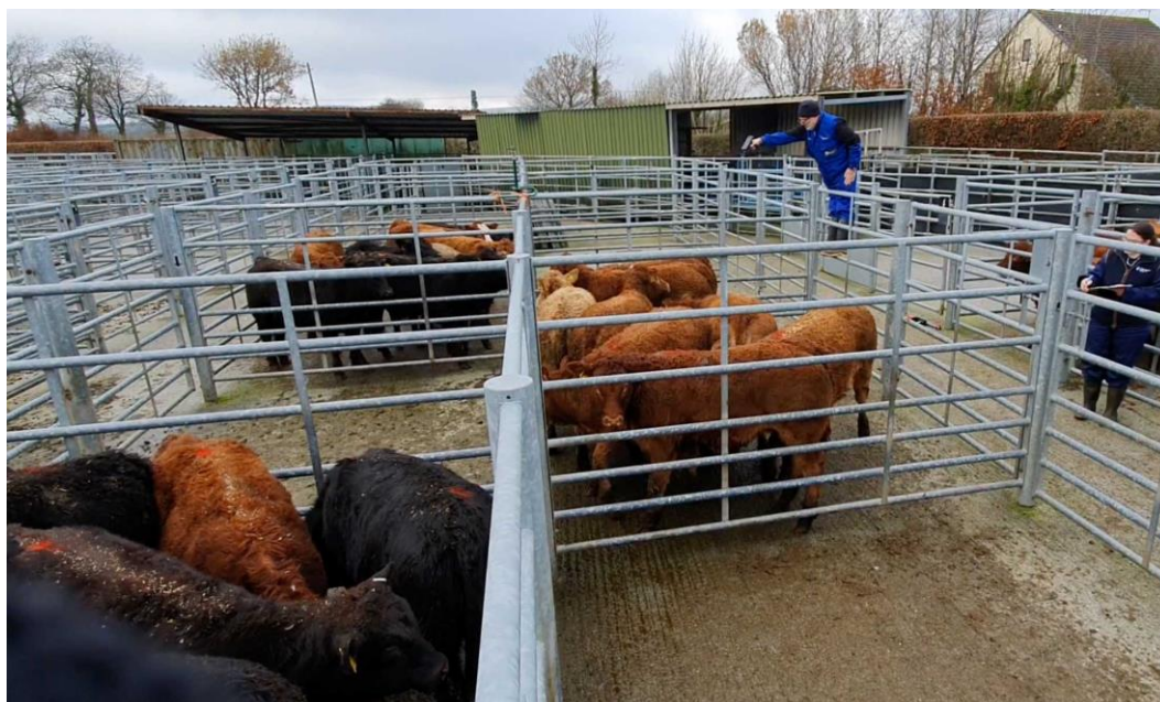
Figure 3.5. The pen with the target animals (on the right) being scanned with the UHF hand-held reader in pen test 2. Note that the operator is trying to use the scanner as high as possible to avoid scanning non-target animals in other pens and to scan 'over' animals in front of them to read those behind.
