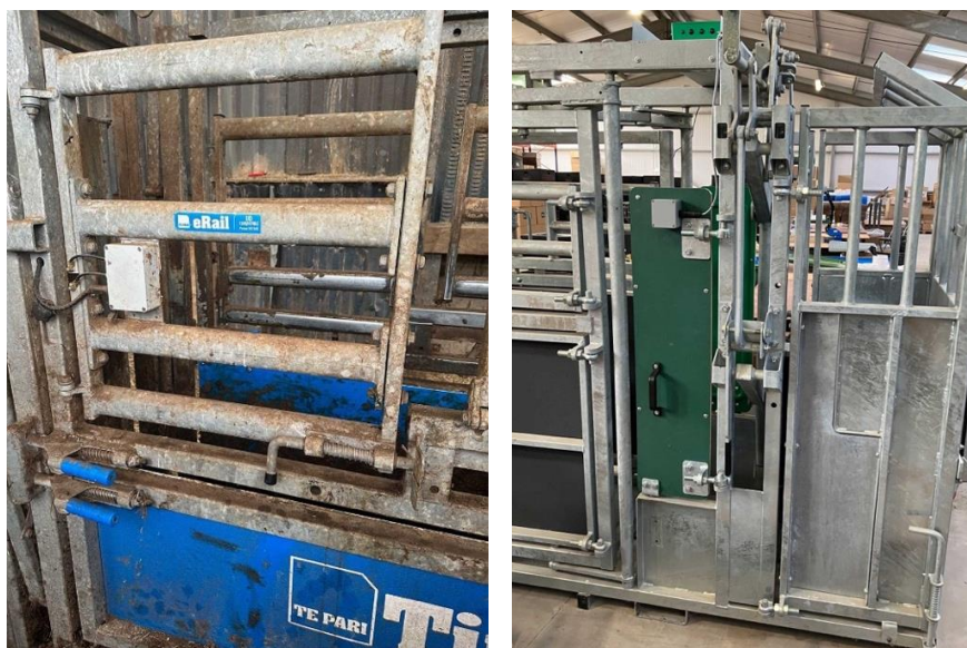
Figure 6.1. Photographs showing two options for incorporating EID panels into crush doors. These maintain the operational functionality of the crush (i.e. the doors still work as before) whilst ensuring the LF antennas are well placed to read the ear tag of an animal standing in the crush.
