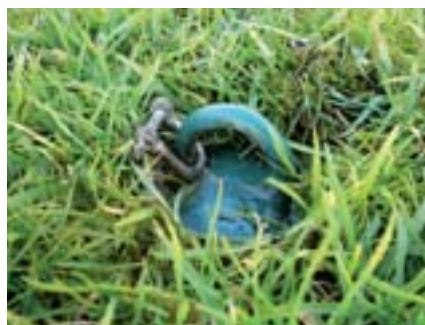
Corkscrew anchor in position.
