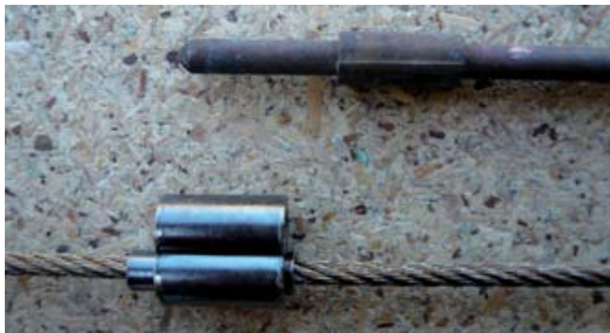
Copper wire tealer (top) and (below) the snare cable showing one style of tealer-clip. Note the collar on the tealer which prevents the clip sliding down.
