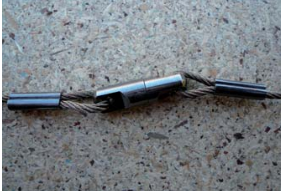
A quality mid-point swivel: small, strong and rotates easily under strain.
