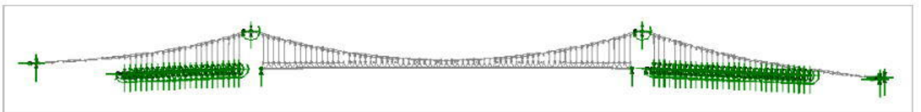
Figure 13: External boundary conditions. Note the back span viaducts and main towers are not modelled; these are represented by fixed translational and rotational supports
