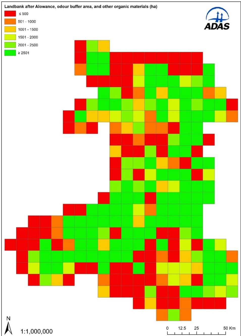
Figure 17. Final landbank (ha). No application to slope >12°, 10 m buffer around surface water and 50 m around boreholes, springs and wells, 50 m urban/odour buffer, organic material restrictions in SPZ1, designated sites, land under Glastir management and according to soil pH and metal concentrations. Accounting for applications of livestock manures, compost, digestate, biosolids and wastes applied under Environmental Permitting Regulations. Total available landbank is 579,000 ha. One grid square = 10,000 ha.
