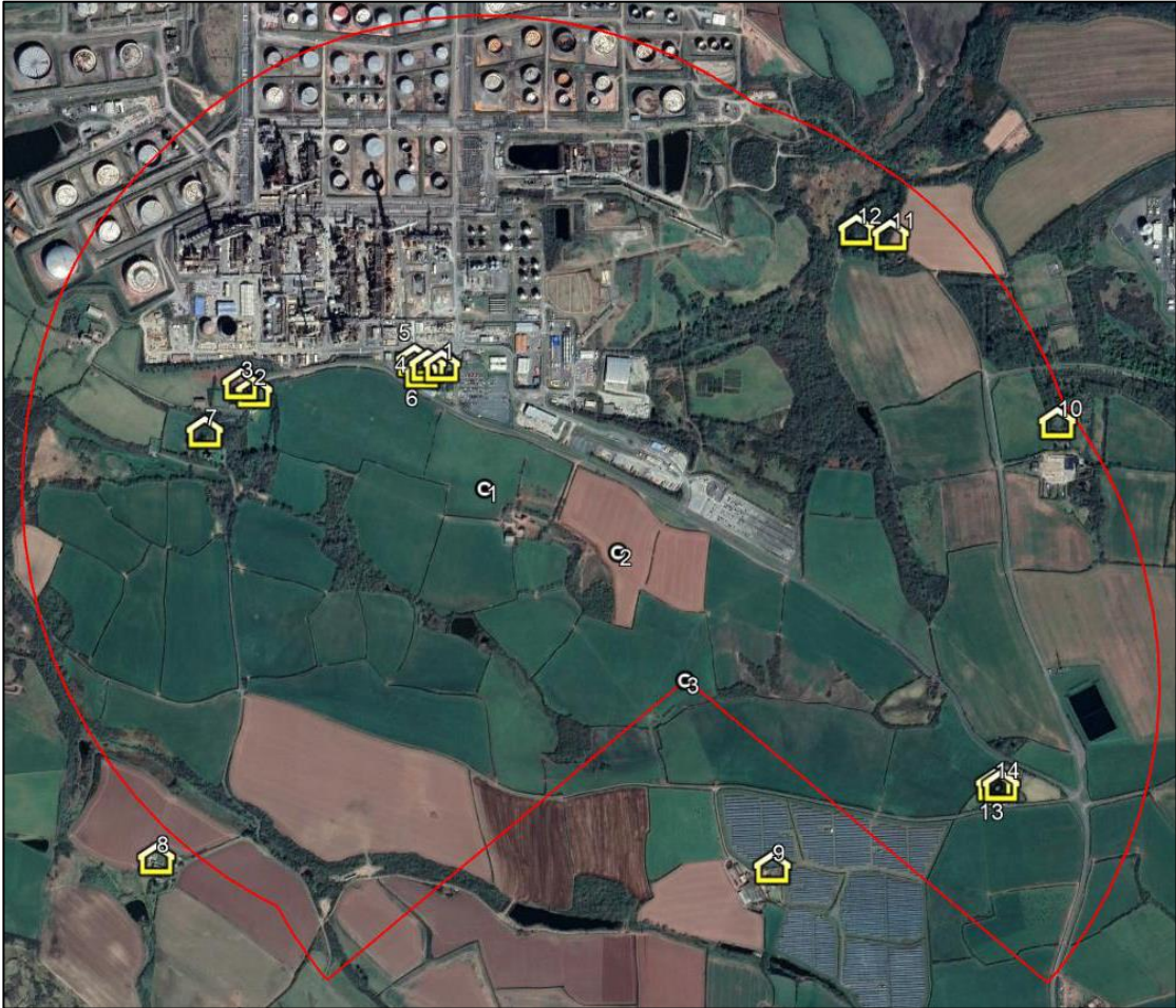
Figure 3 All identified receptors relative to the 10 rotor diameter zone and cumulative 130° either side of north zone
