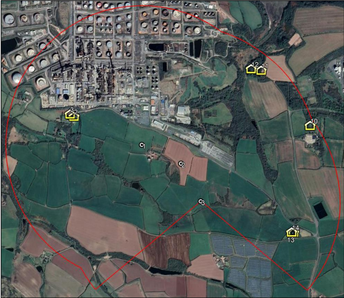
Figure 4 Identified receptors considered for the assessment relative to the 10 rotor diameter zone and cumulative 130° either side of north zone
