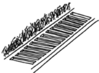
Drains should be fitted to the pitch to make sure it does not flood.
