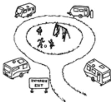
The ‘circular’ (also known as loop or horseshoe) design has a shared entrance and exit with a looped road. Trailers are placed around the loop. A play area is usually in the centre.
