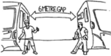
A gap of 3 metres should be kept between trailers and the edge of the pitch. Caravans should not be less than 6 metres from any other caravan. This is to prevent fires spreading between caravans.
